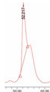
Figure 7. Typical chromatogram from semipreparative HPLC separation of the Mosher ester (3 S ,7 S ,11 R ,15 S )-21 S . The shoulder on the tail of the main peak is the C3 epimer (3 R ,7 S ,11 R ,15 S )-21 S .
